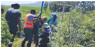
Installing a deep piezometer (Photo: AT Grundling)
